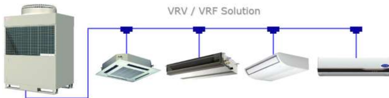
VRF system Outdoor and Indoor units – One Outdoor Unit Serves Multiple Indoor Units.
